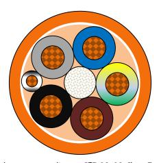
Flexible bare copper conductors according to CEI 20-29 Class 5 and DIN-VDE 0295 K5 Construction:
