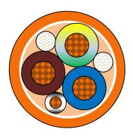
Construction: Flexible bare copper conductors according to CEI 20-29 Class 5 and DIN-VDE 0295 K5
