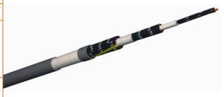
PVC PUR, class 6 conductors, drag chain power and control cable for application in drag chains for short and medium distances, and medium and high speed of movements.
